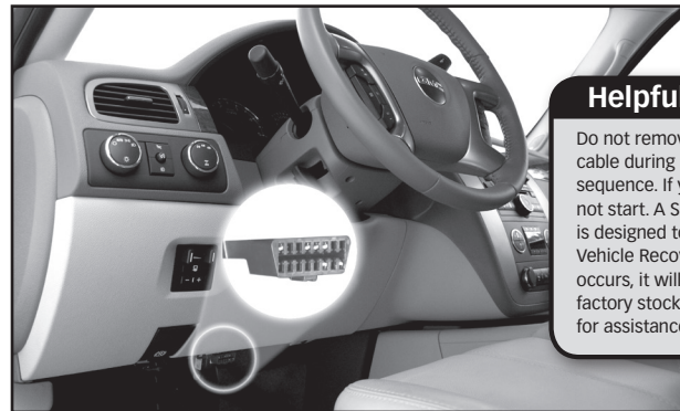
Your OBD-II Vehicle Port is usually located under the drivers side dash as shown here.
